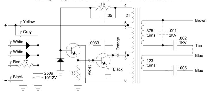
It appears that the circuit was designed to have power applied to the Red lead with the Grey & Yellow leads connected, possibly through a control switch or relay, in which case the supply voltage would have been less than 10 volts due to the 250u 10/12V capacitor.
